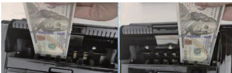
Figure 7-16 One banknote to Check the Gap between the Rollers
