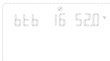
Figure 1-30 Setting of battery voltage point when mains switch back to battery mode
